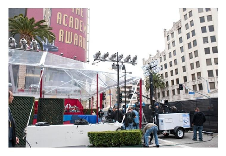
This prototype mobile lighting unit, which uses energy-efficient lighting and hydrogen fuel cell power, was used during the Academy Awards. Its backers hope similar technologies can replace noisy, polluting diesel-based mobile lighting. | Photos courtesy of the Academy of Motion Picture Arts and Sciences®
