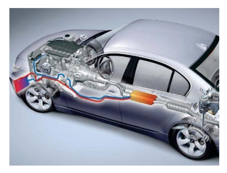
This image shows how a thermoelectric generator would be placed in a passenger car. | Photo courtesy of BMW
